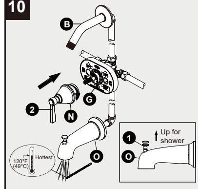
To adjust maximum temperature, go to step 11. If not, go to step 12.
