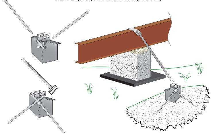
Using a soil test probe, determine the soil classification. Place the X-Plate parallel to the building being secured with the flat plate to the inside. Pound the plate into the ground so that the upper lip is ground level. Using a heavy hammer or electric hammer gun, pound rods into the ground through the box tubing guides welded onto the back side of the stabilizer plate. Rods should be installed until maximum 1" above the box tubing.
