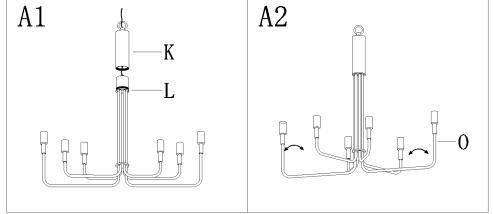
Step A1: Slip tube (K) over the wires and then thread it into the top of fixture loop (L). Step A2: Adjust the arms (O) to the proper position.
