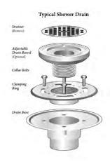
An exploded view of a typical shower flanged drain assembly is shown below. This assembly can be made from PVC, cast iron or other composite materials. Square tile insert drain will replace the strainer only.
