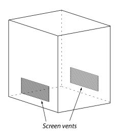
Make sure each opening has a total free area of not less then ½ square inch per pound (3.2 sq. cm/kg) of stored fuel capacity and not less then a total free area of 10 square inches (64.5 sq. cm).
