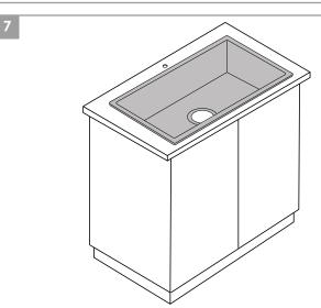
Check alignment of sink again to secure sink. Wipe away excess silicone caulk with damp cloth. Connect drain and water supply according to manufacturer's instruction.
