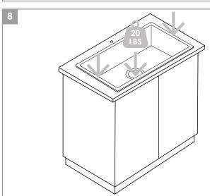
After sink is positioned on set on countertop, it is recommended to wait for 24 hours to allow silicone adhesive to cure, also keep at least 20 pounds weight on the sink to ensure full sealing and curing of the silicone on the whole mounting flange.
