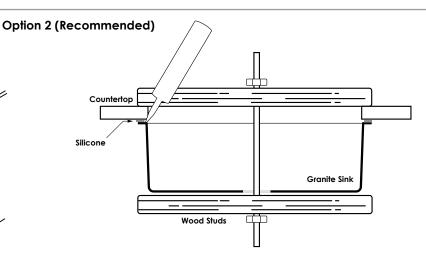
Clamp the boards so the sink stays suspended about 1 in below the countertop. Clean sink flange and underside of cut-out area of countertop, making sure that the area is smooth and free of debris. Apply continuous bead of silicone caulk evenly on top of sink flange.
