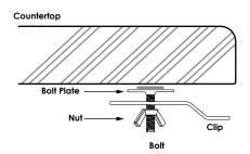
Distribute clips evenly around sink cut-out, determine where to glue the bolt plates. Stick bolt plates under the countertop and let adhesive to cure before applying any weight.
