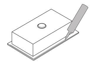
Clean sink flange and underside of cut-out area of countertop, making sure that the area is smooth and free of debris. Apply continuous bead of silicone.
