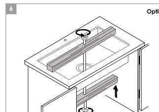
Clamp the sink and hold in place while adhesive cures. There are different methods, we suggest using a couple of pieces of wood with a threaded rod. Set one piece of wood under the sink and another over the countertop.
