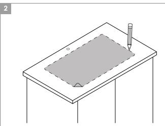
Place cut-out template in desired position on countertop locating center of the bowl over cabinet.
