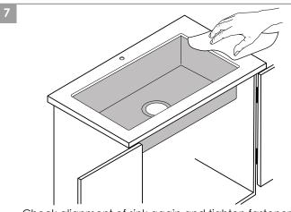
Check alignment of sink again and tighten fasteners to secure sink. Wipe away excess silicone caulk with damp cloth. Connect drain and water supply according to manufacturer's instruction.
