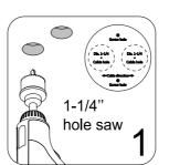
Reference steps 1-2 of surface mount section to turn off power source and separate puck from trim ring. Then use reference template to drill 2 pilot screw holes. Use a hole saw to drill two 1-1/4'
