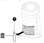
3 Slide the filter out and remove it from its packaging.
