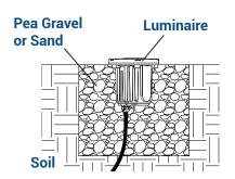
Install the fixture in the hole and fill it with pea gravel or sand.
