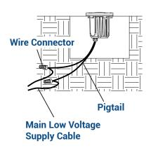
Strip both leads from the fixture pigtail. Using two wire connectors (sold separately), connect the leads from the fixture to the main low voltage supply cable leads.
