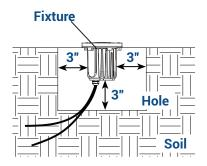
Dig a hole in the ground. Make sure there is approximately a 3" space surrounding all sides of the fixture housing for pea gravel or sand.
