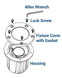
Place the fixture cover with the gasket onto the housing and secure them with the lock screws. Hand tighten with Allen wrench
