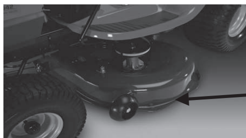
Stamped Deck Shell below, NOT reinforced
