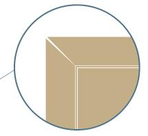
When wood swells, miter joints open as shown above.
