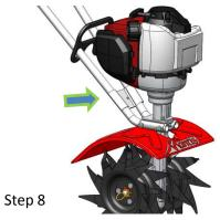
Lean the Tiller Handles against a sturdy surface, so the tiller is supported in the upright position. Place the Top Bracket over the Lower Handles and below the Carry Handle.
