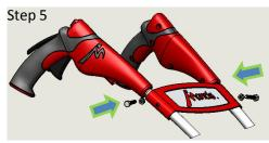
Line up the Handle Brace with the holes on the Upper Handles. Insert cap screws **T15** through the holes in the Handle Brace and through the holes on the Upper Handles. Secure with a lock nut **T14**.
