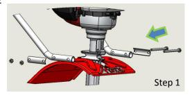
Slide two (2) **T11** bolts through the holes of one Handle Clamp and then through the holes of the Left Lower Handle. Position the bolts so that one bolt is in front and one bolt is behind the recessed channels of the transmission housing. Slide the Right Lower Handle and the second Handle Clamp onto the bolts. Finger tighten the nuts **T14**.
