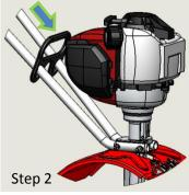
Slide the Carrying Handle over both Lower Handles. Slide it down towards the engine. It will rest about four to six inches above the engine.
