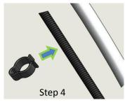
Use the clip **T9** to secure the throttle cable and wire in place on the Right Lower Handle.
