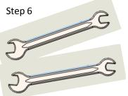
Tighten all lock nuts, cap screws, and bolts firmly and securely using two 7/16" wrenches.
