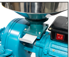
8. Lay the iron sheet and the discharge port, screw on the screw and complete the installation
