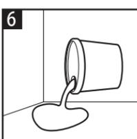
8. Prime subfloor with latex based flooring primer (not included). Primer must be of type specifically designed for use with self-adhesive (self-stick) vinyl flooring. Follow manufacturer's directions for proper application and mixing of flooring primer.
