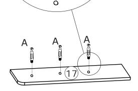
Insert quickfit screw(A) into plate 17 with a screwdriver as shown.
