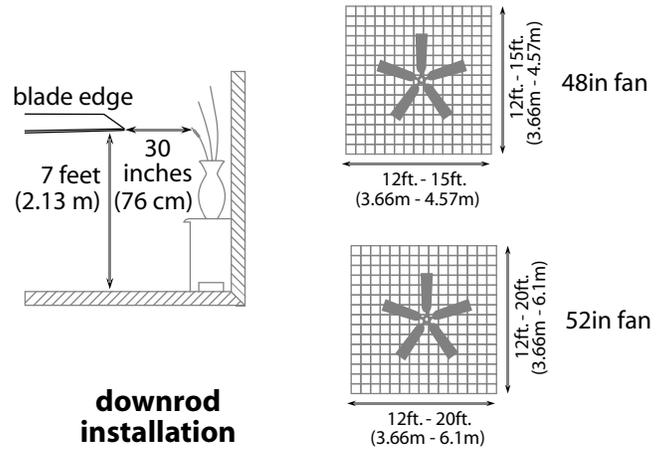
This fan can be mounted with a **downrod** on a regular (no-slope) or vaulted ceiling. The hanging length can be extended by purchasing a longer downrod (0.5in./1.27cm diameter). Other installation, such as **flushmount**, is *not* available for this fan.
