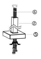
2. Screw and hand tighten the water supply hoses to the subject(DO NOT USE SPANNER TO TIGHTEN AS IT CAN DAMAGE THE O-RING). Make sure the water supply hoses were screwed into the correct inlets for hot water and cold water.
