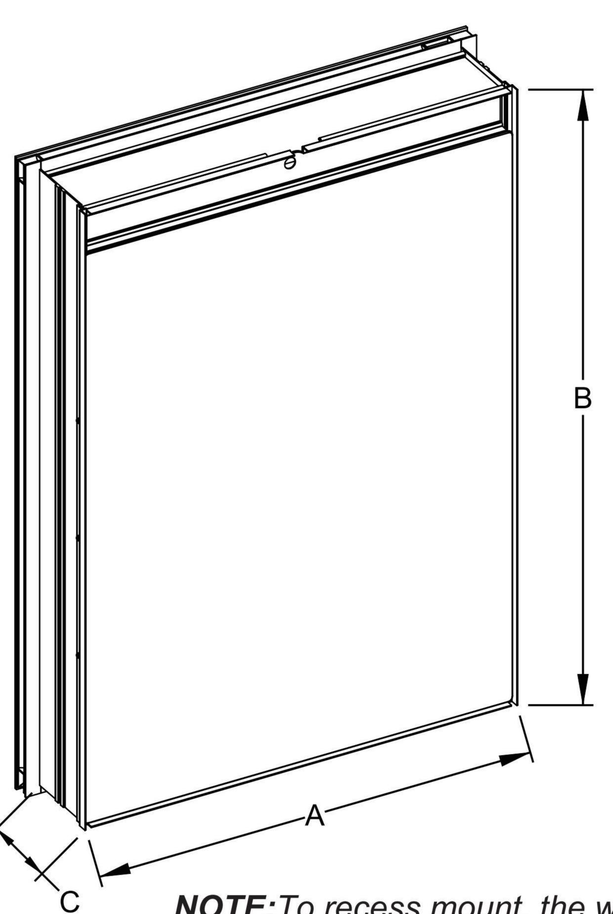
NOTE: To recess mount, the wall cavity must be framed and the cabinet secured to framing studs. Reroute electrical or water supply lines from the cavity. Consult a professional if drain or vent piping is encountered, or if the wall is load-bearing.
