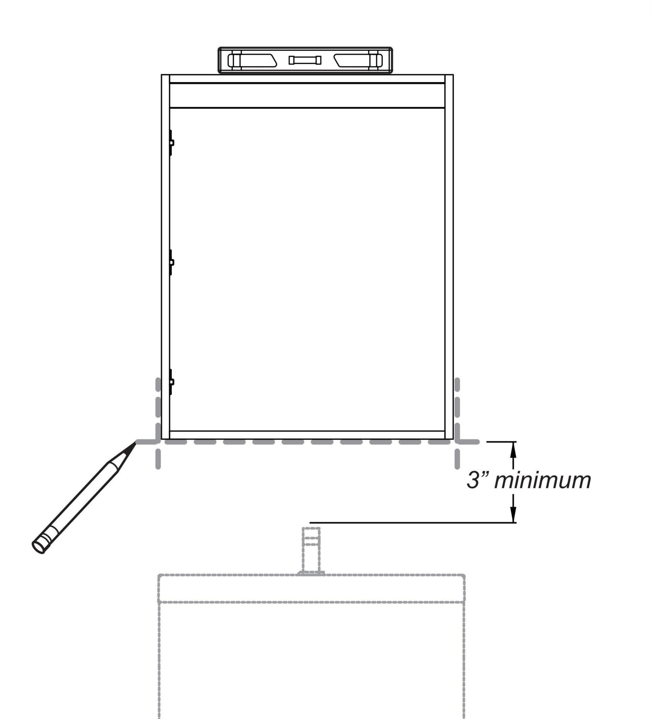
Mark the position of the Bottom Mounting Bracket and Punch.
