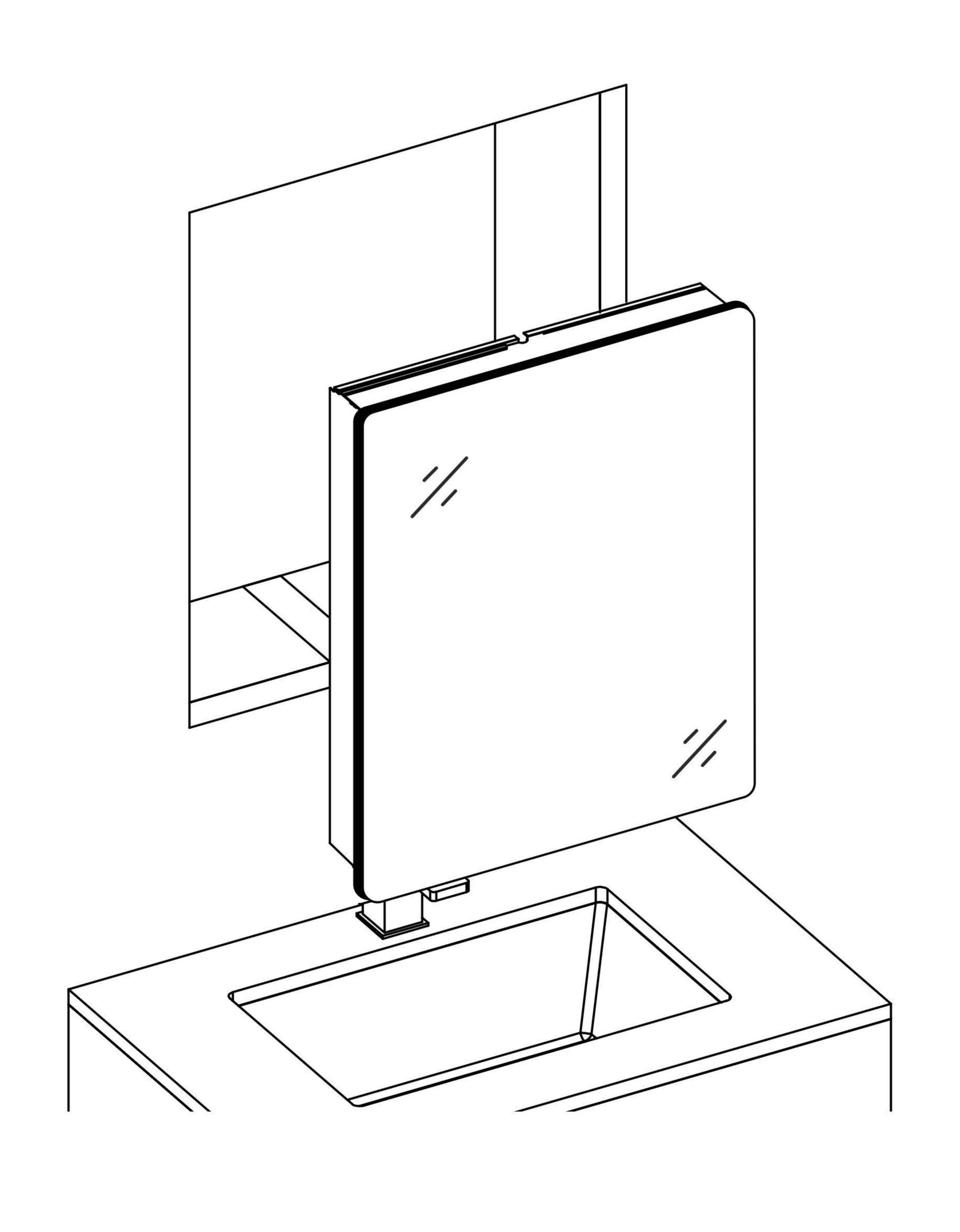
Affix using hardware screws into the studs.
