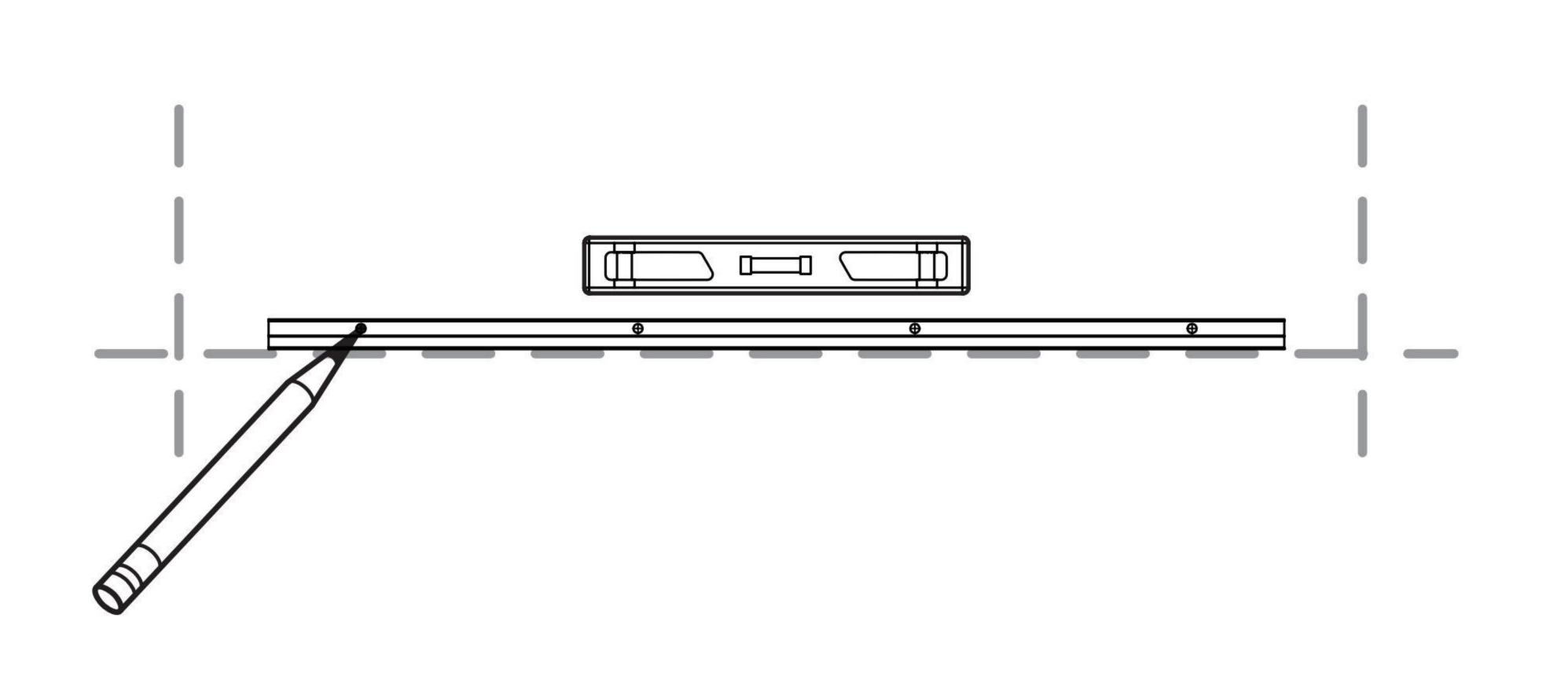
Bottom mounting brackets must be attached to furring strip/channel or wall studs
