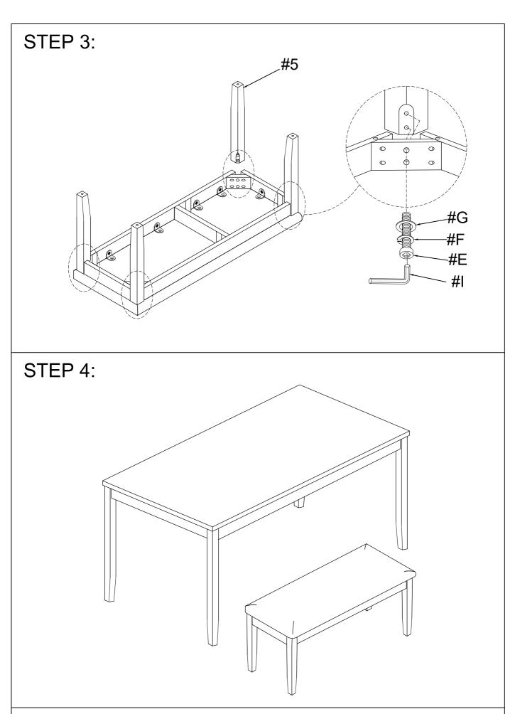
Tighten all screws until completely asembled.
