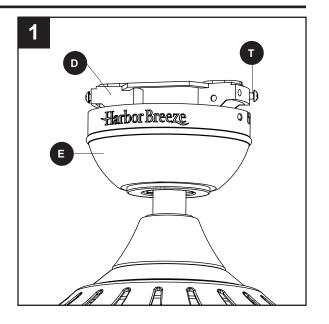
Secure the canopy (E) with the mounting bracket screws (T) previously removed (Step 4, page 8). Tighten all mounting bracket screws (T) securely.
