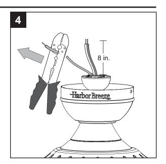
If you decided to cut back the lead wire in Step 4, strip 1/2 in. of insulation from the end of the white wire. Twist the stripped ends of each strand of wire within the insulation with pliers (not included). Repeat the step for black and blue wires.
