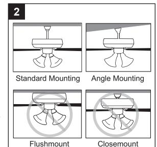
Ensure the blades (S) will be at least 30 in. from any obstructions. Also check the downrod (A) length to ensure the blades (S) will be at least 7 ft. above the floor.
