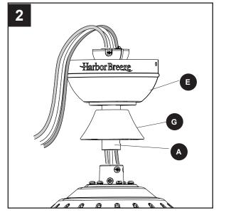
Slide the downrod (A) into the yoke, align the holes, then re-install the downrod pin (B) and downrod clip (C). Secure with set screws (I) and slide the yoke cover (G) down until it rests on top of the motor assembly (H).
