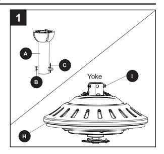
Insert the downrod (A) -- or a longer downrod, if required -- through the canopy (E) and yoke cover (G). Feed the wires from the fan through the downrod (A).
