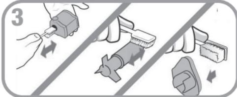
**Step 3.** Use a soft cloth or brush and warm water to clean the impeller and the inside of the impeller housing.
