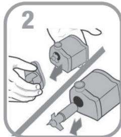
**Step 2.** Remove the impeller cover to expose the impeller assembly. Remove the impeller assembly by gently pulling on the impeller blades. The impeller is held in place by a magnet.
