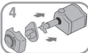
**Step 4.** Reassemble all pump parts and place in water before reconnecting to the power source.
