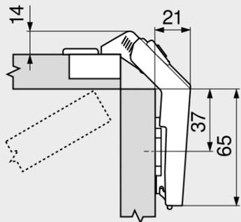
Application type for front thickness FD 19 mm in conjunction with 0 mm spaced standard mounting plate
