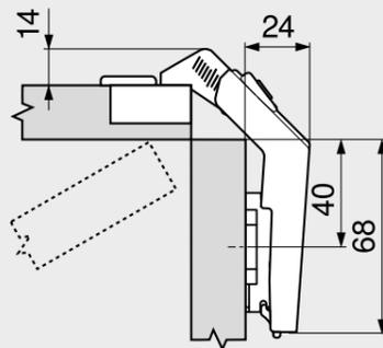
Application type for front thickness FD 19 mm in conjunction with 3 mm spaced standard mounting plate
