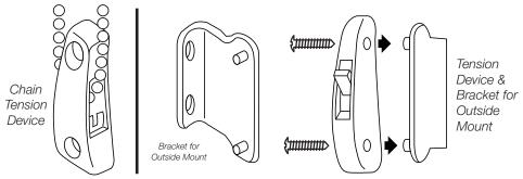
Inside Mount: if mounting into wood, pre-drill screw holes and then install the tension device using the 11/4" Phillips head screws provided.
