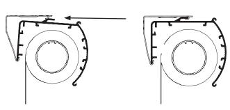
Snap Headrail into place by sliding groove in back of headrail into the bottom of the mounting bracket. Push forward and up, snapping the headrail into the top of the mounting bracket.
