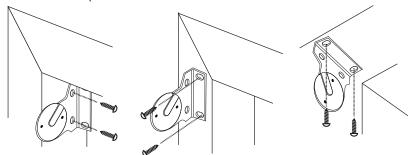
Mark the screw locations with a pencil - pre-drill the screw holes using a 5/64" drill bit.
