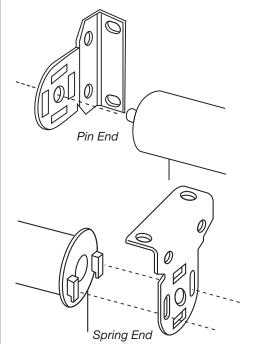
**Step 2A.** Cassette Installation (for shades with optional Cassette Valance) The shade is pre-mounted in the cassette. It can be removed to adjust tension, if necessary.
