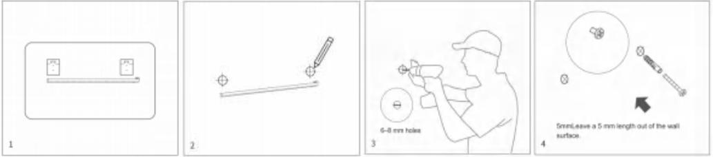
1. Measure the hanger spacing Measure the distance between 2 hangers with a tape measure
