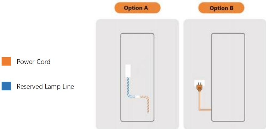
Cut out the plug and the reserved wire connection port, which can be hidden on the back of the mirror
