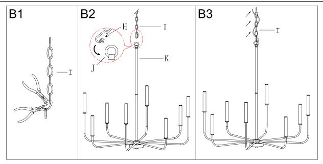
Step B1 » By measuring, determine the correct number of links needed for proper hanging height. Using the chain pliers, disconnect and discard the unwanted part.
