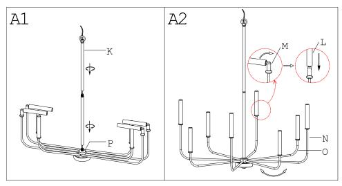
Step A1 » Screw tubes (K) onto top of arm assembly (P) as shown in the illustration.
