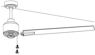
Remove the pre-installed screws.
