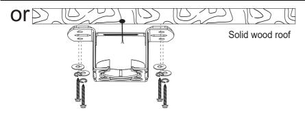
(3) Snap the basically assembled fan into the installed Bracket.
