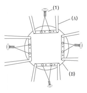
Secure Legs (A) to Seat (B) with Allen Key Screws (1). Use Allen Key (2) to tighten. Do not over-tighten.
