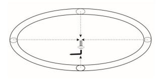
Remove the Allen Key Screws (1) from Foot Ring (C) using Allen Key (2).
