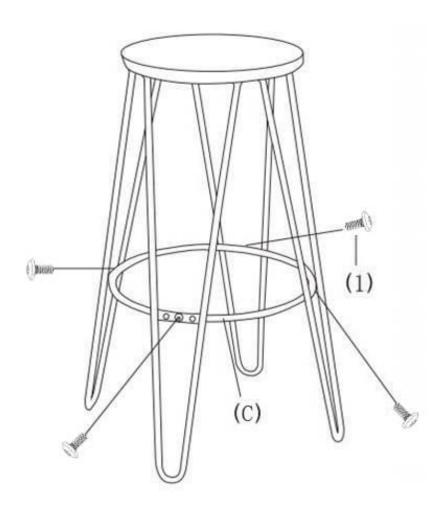
Attach Foot Ring (C) to Legs (A) with Allen Key Screws (1). Use Allen Key (2) to tighten all screws.
