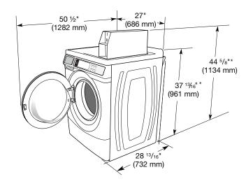
\*Height without leveling feet installed
