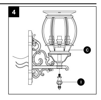
5. Place fixture (C) onto mounting screws on crossbar (CC). Re-attach rings (DD) and secure with cap nuts (EE).
