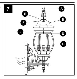
Note: Before use, add silicone glass sealant between wall and canopy, leaving the bottom clear so moisture can drip down.
