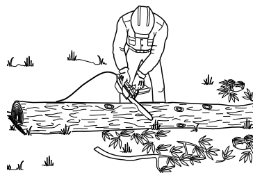
Figure 14 - Bucking Log With Entire Length On Ground
