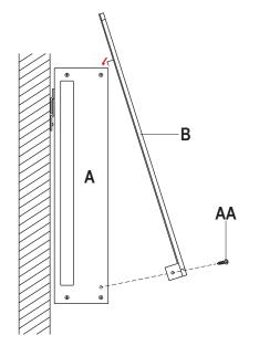
Lift Glass Front (B) into place, ensuring the 2 tabs on the top backside of the glass fit securely into the holes on the top of Firebox (A).
