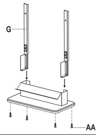
**2** Attach the left and right Tabletop Supports (G) to the table top base (J) using 4 screws (AA).
