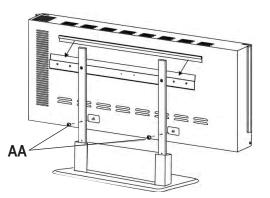
4 Hang Electric Firebox (A) on Mounting Bracket (C). Secure the Firebox (A) to Mounting Bracket (C) with two M4x8mm Screws (AA).
