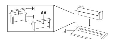
Attach Deflector (H) to Front (I) using two M4x8mm Screws (AA).
