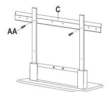
Secure Mounting Bracket (C) to the tabletop stand with two M4x8mm Screws (AA).
