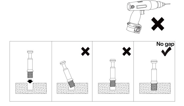
Screw the pin into the hole. Set the cams correctly by aligning the head of the cams with the lock pins.Lock the cam by turning the cam head with a screwdriver until it istightened. Please do not use an electric screwdriver to assemble the unit.
