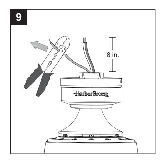
If you decided to cut back the lead wire in Step 9, strip 1/2 in. of insulation from the end of the white wire. Twist the stripped ends of each strand of wire within the insulation with pliers (not included). Repeat this step for the black wire.
