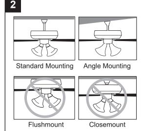
3. Ensure the blades (Q) will be at least 30 in. from any obstructions. Also check the downrod (A) length to ensure the blades (Q) will be at least 7 ft. above the floor.
