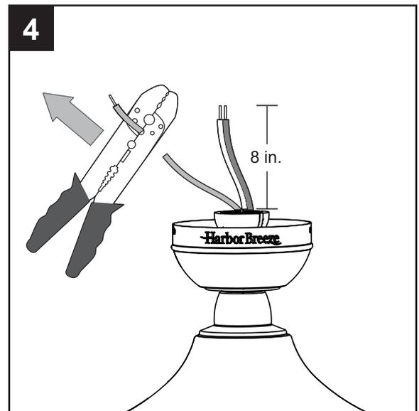
5. If you decided to cut back the lead wire in Step 4, strip 1/2 in. of insulation from the end of the white wire. Twist the stripped ends of each strand of wire within the insulation with pliers (not included). Repeat the step for the black wire.
