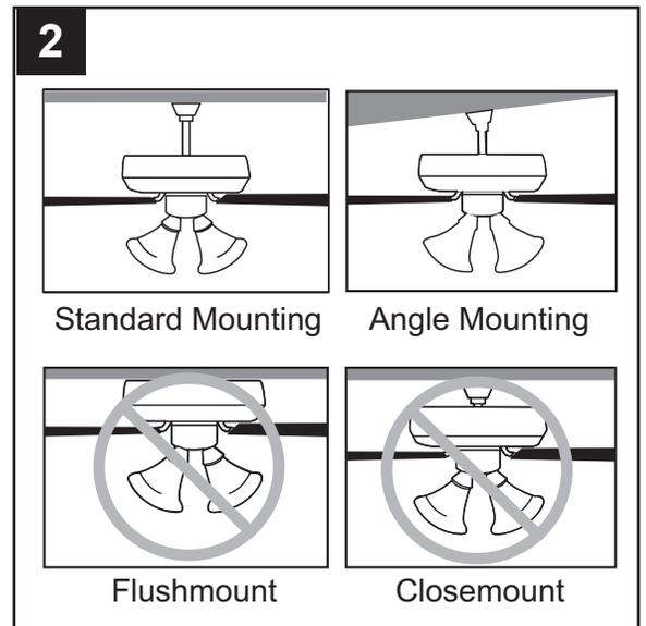
3. Ensure the blades (L) will be at least 30 in. from any obstructions. Also check the downrod (A) length to ensure the blades (L) will be at least 7 ft. above the floor.
