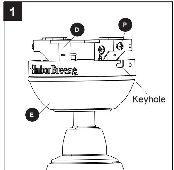
2. Secure the canopy (E) with the mounting bracket screws (P) previously removed (Step 4, page 8). Tighten all mounting bracket screws (P) securely.
