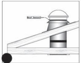
[14] Fasten flashing to the tube assembly with 4 #8 x 3/4" sheet metal screws provided in kit. [15] Caulk around the tube, at the roof jack and the vertical seam of the tube. [16] Apply the storm collar to the tube, just above the roof jack flashing. Caulk around the top of the storm collar.
