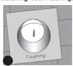
Center flashing over screw, trace inside diameter onto roof shingles
