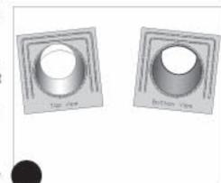
Apply roof sealant to top and bottom of flashing as shown
