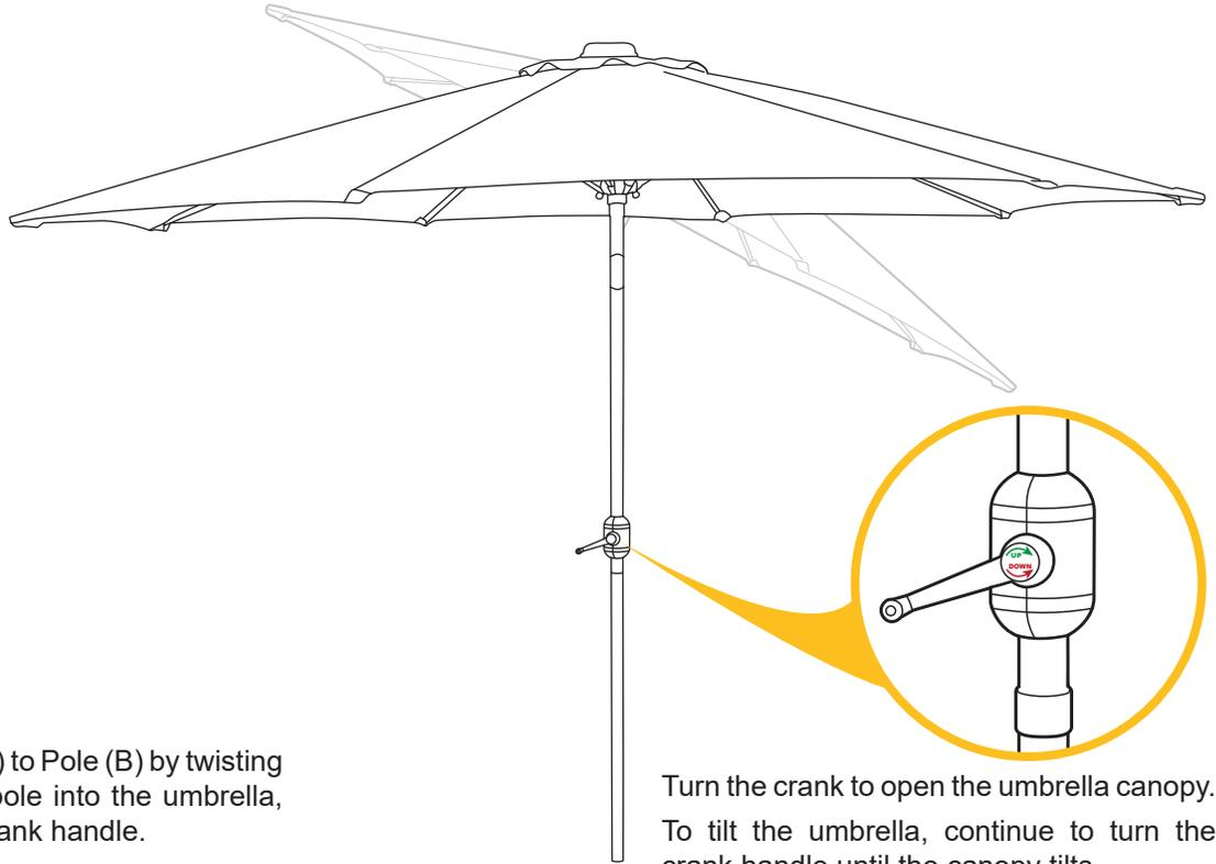
Turn the crank to open the umbrella canopy. To tilt the umbrella, continue to turn the crank handle until the canopy tilts.
