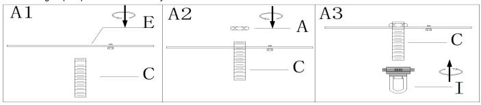
Step A1: Thread the single bar(E) onto nipple (C), At this point need note that: the side of single bar marked "GND" must
