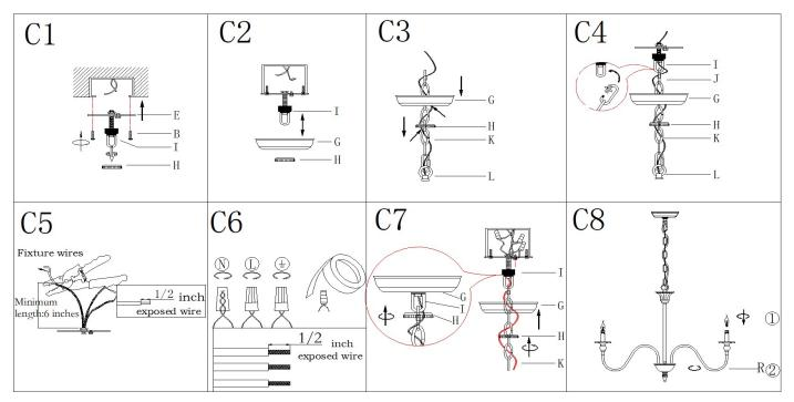
Step C1: .Attach the single bar (E) to outlet box with mounting screws (B). The side of single bar marked "GND" must face out Step C2: Pass canopy (H) over the mounted collar loop (I) then secure with threaded ring (H) to test the height .Unscrew
