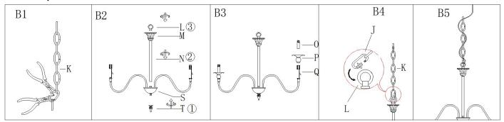
Step B1: By measuring, determine the correct number of links needed for proper hanging height. Using the chain pliers, disconnect and discard the remaining chain.
