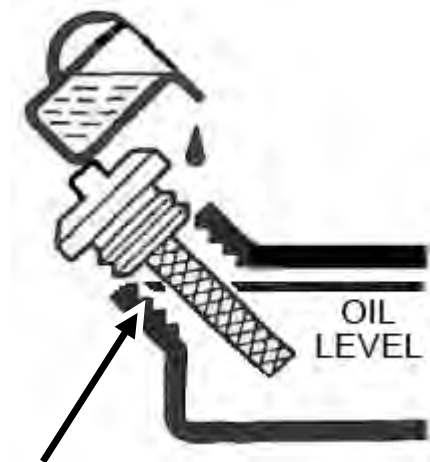
Figure 2 - Add Oil To TOP Of Threads
