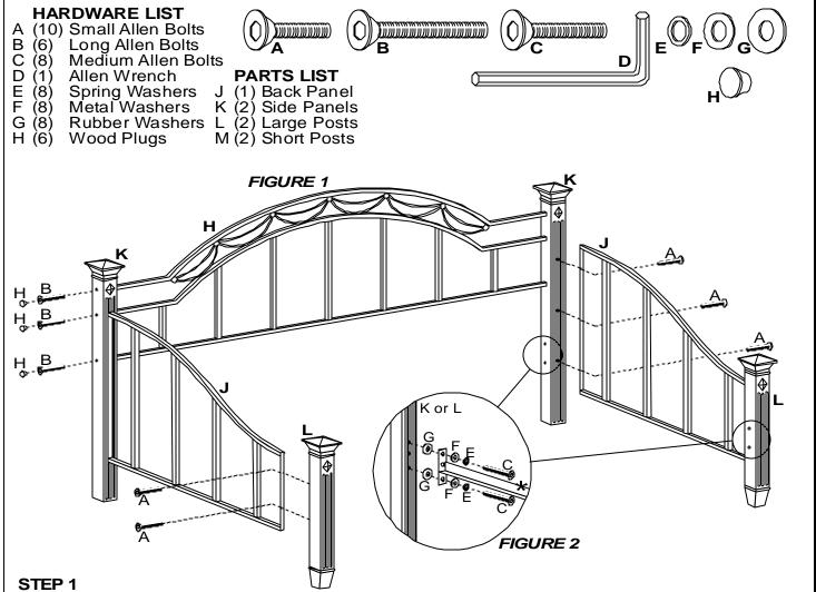
Begin assembly by both Large Posts (K) to Back Panel (H), using 3 Long Allen Bolts (B) per each side. Only tighten bolts by hand for this step. See Figure 1.
