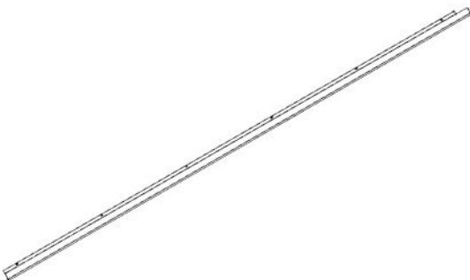
G01 LEFT GUTTER 10FT - A4M03478 (x1) 1 9/16"x1 15/16"x1117 5/16" (40x50x2838)
