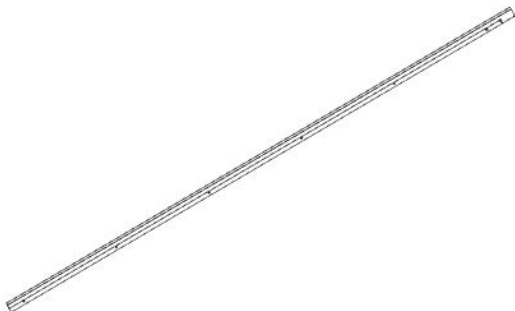
G02 GUTTER - A4M03481 (x1) 1 9/16"x1 15/16"x1117 5/16" (40x50x2838)
