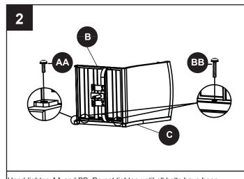
Hand tighten AA and BB. Do not tighten until all bolts have been
