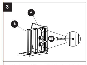
Hand tighten BB. Do not tighten until all bolts have been installed.
