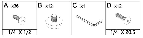
When the process of product assembly, please do not lock the screws at one time, but wait until all the screws are assembled to the position, and then straighten and flatten the product, and then tighten the screws of the same height in turn, so as to avoid unsmooth assembly and product tilt.
