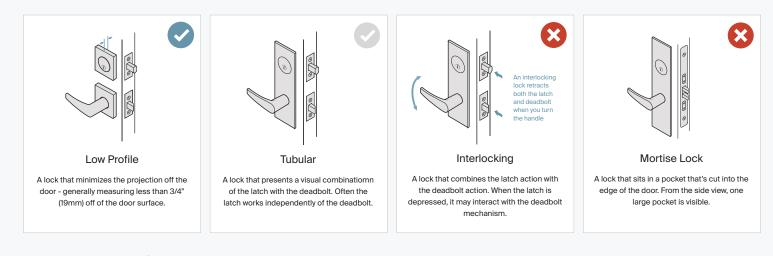
Most Standard and Low Profile residential deadbolts can be replaced with Level Lock.
