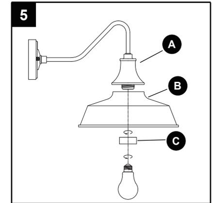
**CAUTION:** To avoid any waterproofing problems, please make sure the light fixture fits the mounting surface perfectly installation and use waterproof glue around the canopy for better sealing after installation.
