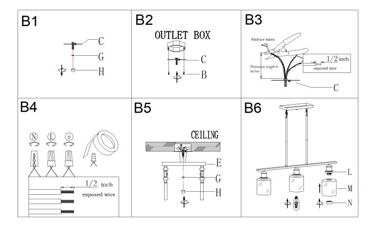
Step B1: Unscrew hex nut (G) and cap nut (H) from single bar (C).
