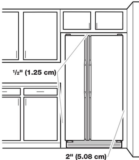
To ensure proper ventilation for your refrigerator, allow for 1/2" (1.25 cm) space on each side and at the top. When installing your refrigerator next to a fixed wall, leave 2" (5.08 cm) minimum on each side (depending on your model) to allow for the door to swing open. If your refrigerator has a water dispenser and ice maker, allow extra space at the back for the water line connections.
