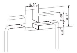
2. The depth of the embedded box is 1.8"-2.2". It's better to drill the depth of 1.8" for blank wall.
