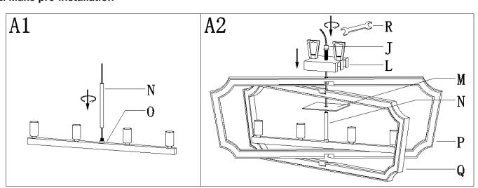
Step A1 » Carefully pass the fixture wires through stem (N), then screw stem (N) onto fixture body (O).
