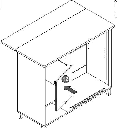
Slant the door 15 degrees and place the pins at both ends into the slots in the cabinet, then place them straight to complete the installation of the door.
