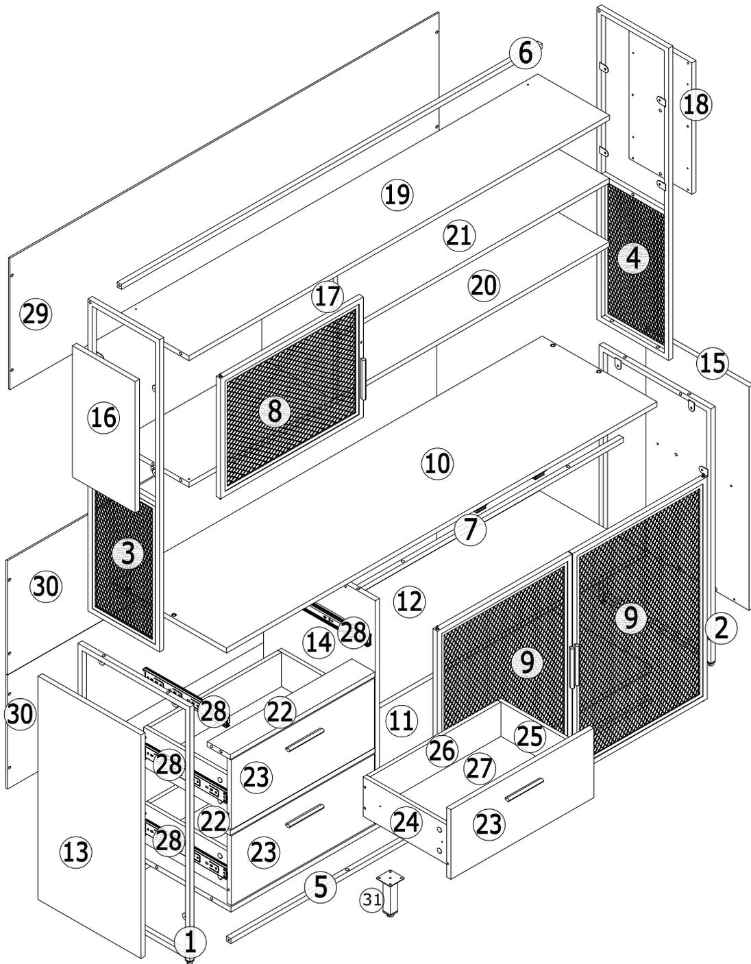
**Slides Must Be Separated Before Assembly.
