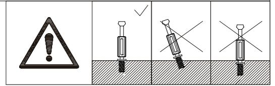
Insert quickfit screw(A)
