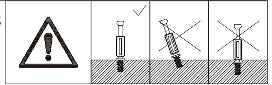
Insert quickfit screw(A) into corresponding holes in board 13 and 15 with a screwdriver as shown.
